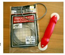
The spline tool is a simple tool with a handle that has a <u>plastic</u> roller at each end. Do not use spline tools with metal rollers, as these will tend to cut the screen material and can easily destroy your screen.
