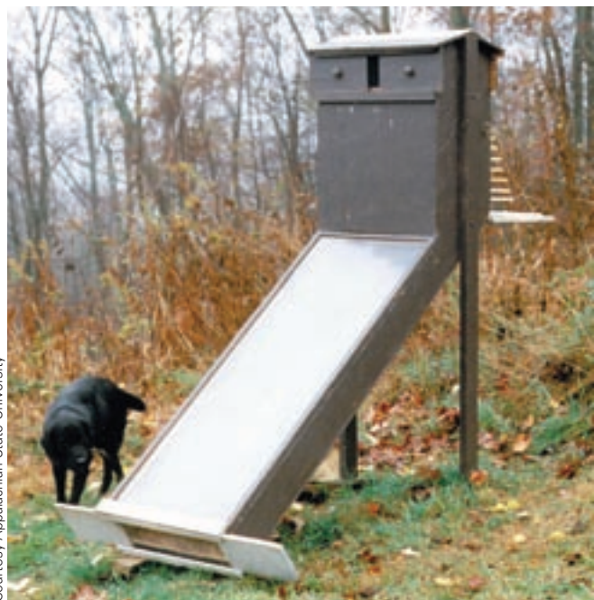
Well-designed through-pass collectors, like this Appalachian Food Dryer, are another solar food dehydrator design option.
